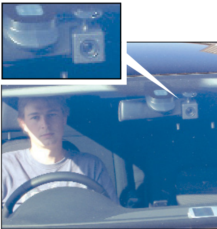
The V1 series camera mounted in front of the rear-view mirror of a vehicle.
